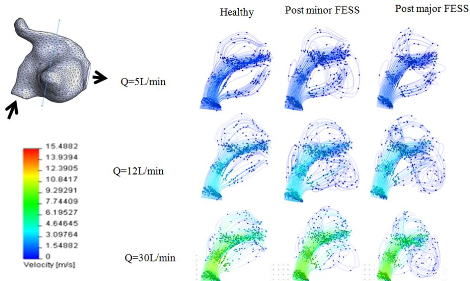
FIGURE 4 Fluid particle trajectory for healthy, post FESS minor and post FESS major actual 3D model.
