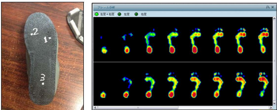
FIGURE 3. Sensor position and load distribution at the time of the walk <sup>[5]</sup>
