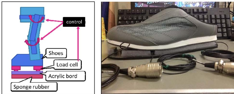
FIGURE 2. Schematic of assist robot and the foot bottom
