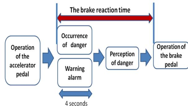
Fig.4 Model of the brake reaction time
