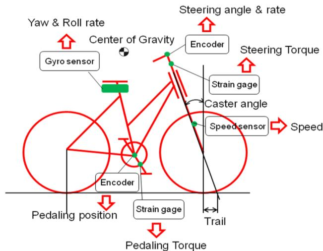
Fig. 4 The measurement system
