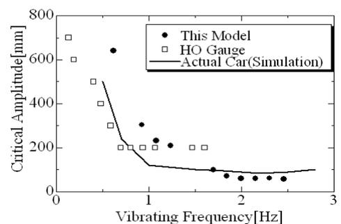
Fig.5 Derailing Limit Curve (After)
