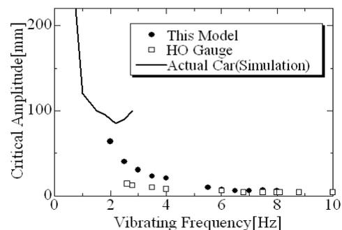
Fig.4 Derailing Limit Curve (Before)
